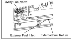
√5 Bleed air from the external tank connecting hose. Fuel can be supplied from the external tank after completing the above procedures.
