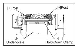
\* Install the battery by performing the above procedures in reverse order. (Always be sure to first attach the "+" (positive) side.)
