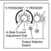
between the middle and maximum positions to enable "1 PERSON" and enable use of the A-side weld outputs for high-current welding. (Refer to section "8-4. Welding Work".)
