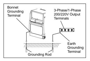
Bonnet Grounding Terminal of this Equipment Perform grounding according to Class D grounding work of the Technical Standards for Electrical Equipment so that the grounding resistance is 100Ω or less. Cable used in grounding must have a thickness that matches the generator capacity.
