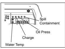
corresponding monitor lamp lights up and the engine is automatically stopped. If the engine is automatically stopped, return the starter switch to "STOP" and restart the engine. Watch the lit/unlit status of the monitor lamps the next time an automatic stop occurs and check the error contents.
