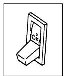
By turning this circuit breaker on the control panel to ON, Power will be transferred to the output receptacles and to the load side.
