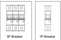
Each receptacle, 3-Phase and 1-Phase is incorporated with circuit breaker respectively. The breaker trips on overload or short-circuit on to stop power transmission to load.
