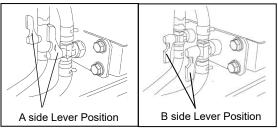
intake and return ports, always turn the lever for 3-way Valve to A position whenever piping work is performed.
