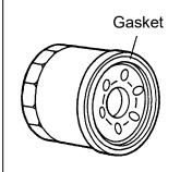
Tighten the Fuel Filter using finger until the filter \_\_\_\_\_\_\_
