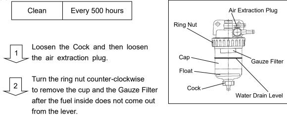
Wash the Gauze Filter in Diesel fuel and reinstall the unit in the reverse order.
