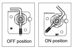
When turning the switch to OFF, the engine electric circuit does not activate due to no battery power.
