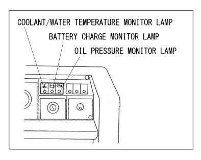
When it is started by the starter switch from STOP to RUN under normal condition, Oil Pressure and Battery Lamps will flash, and then the lamps will go OFF, immediately after the engine starts.
