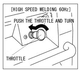
3 Adjust the current by the current adjustment dial. The adjustable current range is different from the throttle position., [Low Speed Welding 50Hz] and [High Speed Welding 60Hz].
