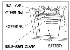
Reinstall a new battery in the reverse order.(Install always the cable to the positive (+) post in the new battery first.)
