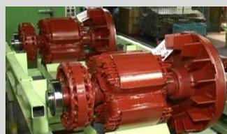
Triple-varnish, standard spec for Shindaiwa's alternator for export, offers robust features of protection against sand gravel, dust, rodent, and burnout including layer short
