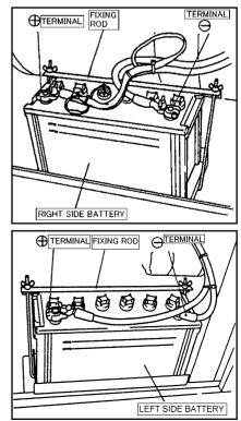
Remove the clamp and cable from **positive (+)** post from the battery on the **left** side.  $\sqrt{5}$ Remove the left side battery from the seat.
